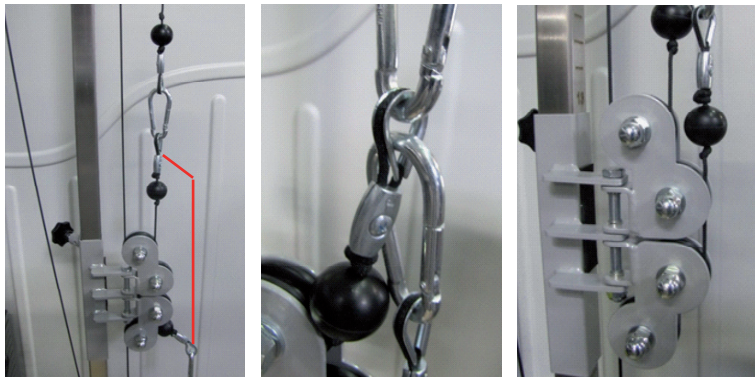
Run the cable upwards through all pulleys
